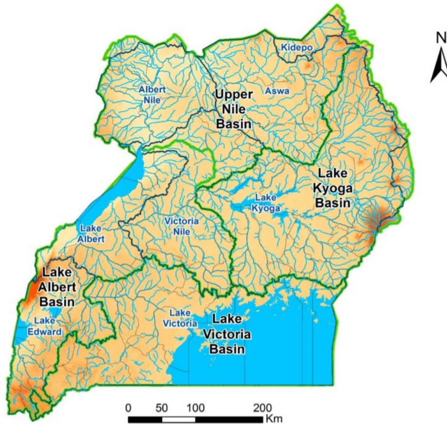
Figure 1: Map of Uganda showing the 4 major basins on whose hydrological flow the Albert, Victoria, Upper Nile, and Kyoga Water Management Zones (WMZs) delineation is based
