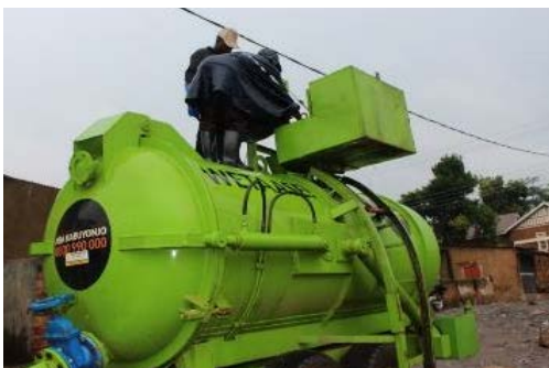
Mobile Transfer Tank
