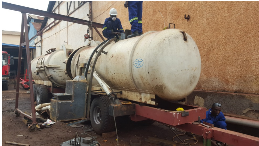
Photograph 4: fabrication of sludge loading system
