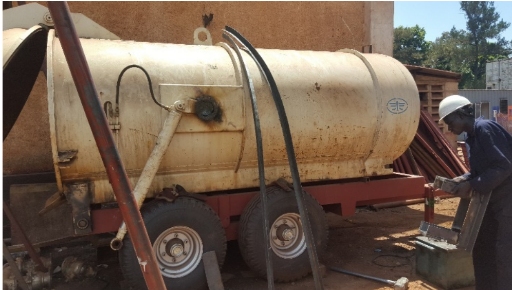
Photograph 5: installing hydraulic systems on the tank
