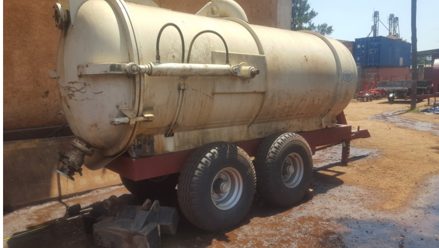
Photograph 3: Mounting tank on new chassis
