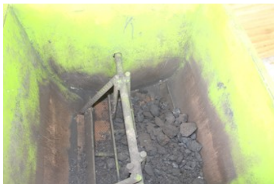
Photo 4: Crushing carbonized char and blended material ready for briquetting
