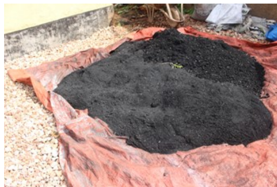
Photo 4: Crushing carbonized char and blended material ready for briquetting
