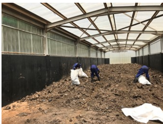
Photo 2: Drying in sludge greenhouse and sludge storage shade
